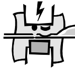
CUT-OFFSEAL 1 x 3,5 mm seal 1 x 1,1 mm cut single time setting
